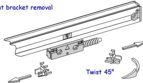
Slide brackets away from reading head and cable.
