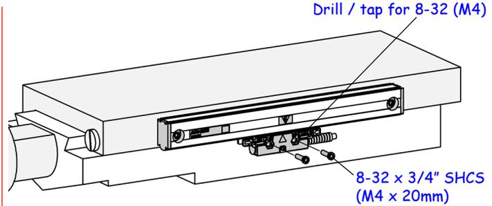
⚠ Do not tighten prior to adjusting leveling set screws
