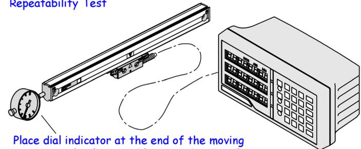
Place dial indicator at the end of the moving component (scale assembly or reading head).
